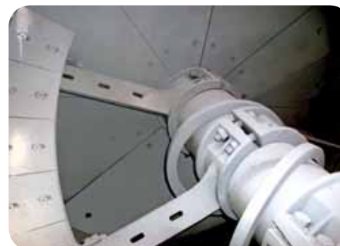
STEEL CAST ARMS, PALLETS WITH DOUBLE SCREW, COVERED SHAFT, RINGS. BRAS EN FONTE, PALETTES A DOUBLE BOULONS, REVETEMENT D'AXE, ANNEAUX
